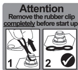
Fig. 2: Information label (red) on the gear unit
