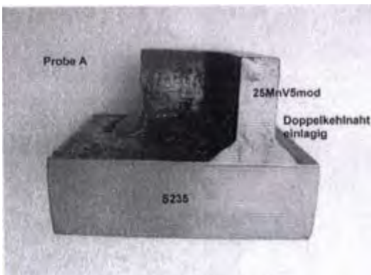
Figure 1: Profile of 25 MnV5mod and S235 single-layered, double-fillet welds
