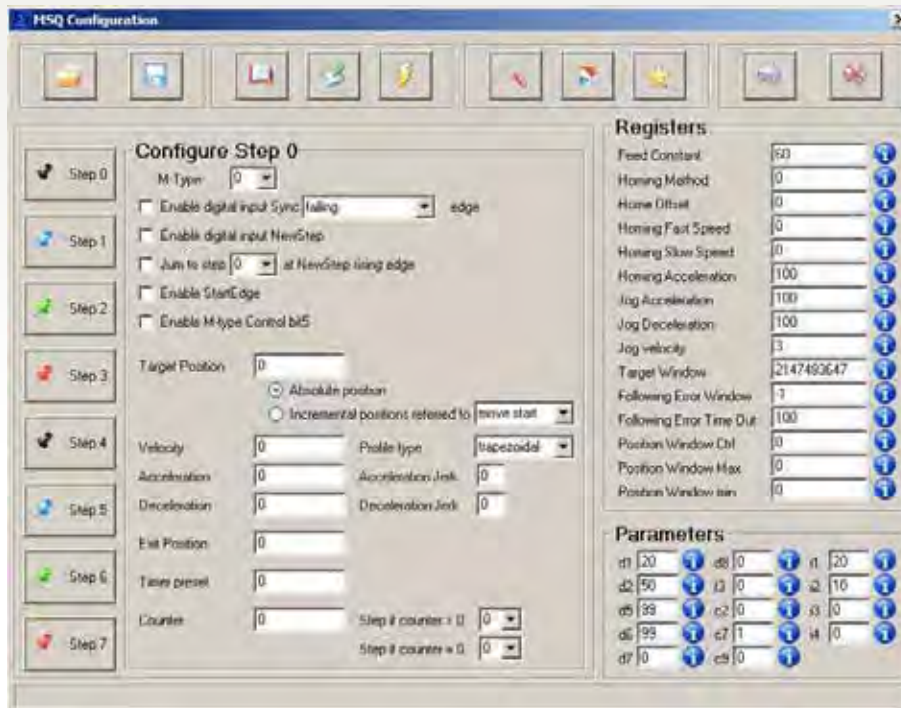
MSQ Control panel
