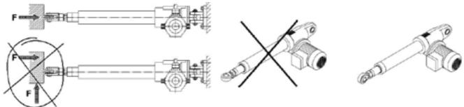
Ball joint front attachment is recommended in case the alignment of front and rear fixing points cannot be guaranteed. An incorrect installation can cause loss of power, malfunctioning, noise and lubricant leakage.
