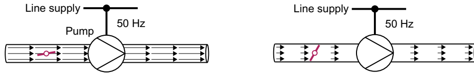
Figure 6-75 Flow control with pump and throttle connected to a 50 Hz line supply
