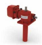
Rotary limit switches can be used as end of travel limit switches, with the option of intermediate switches as well. These units are mounted onto a screw jacks free worm shaft and offer an alternative where bottom pipe mounted limit switches are not possible e.g. rotating screw jacks. Up to 8 limit switches can be accommodated in one enclosure (IP66). Operating temperature -40°C → +80°C.
