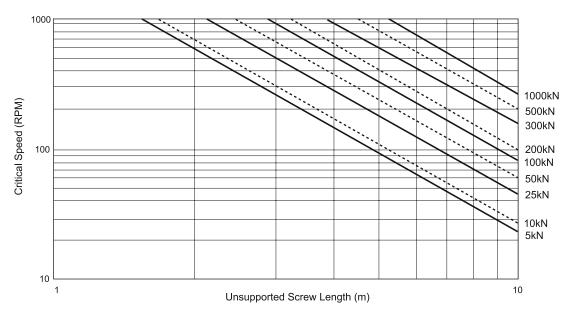
Based on both ends fixed and 80% of the critical speed.
