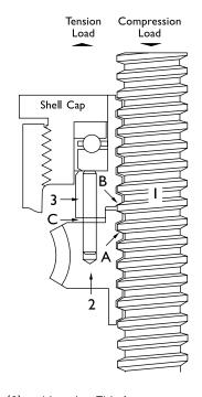
When separation (C) has been reduced to zero, wear has taken place. Replace the worm gear (2) at this point. This feature acts as a built in safety device which can be used to provide wear indication for critical applications.
