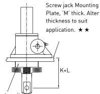
Boot Mounting Plate, to suit collar size. Typically ØB x (E+5 mm fitting allowance) thick.
