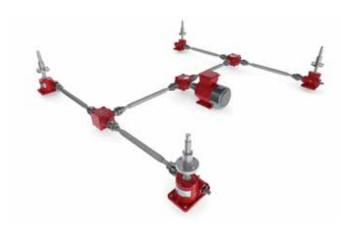
If multiple ball screw jacks are connected in a mechanically linked system then the complete system in some circumstances may be considered self-locking depending on the gear ratios and efficiencies of units in the system. In general, Power Jacks recommend a brake is used on **ALL** Ball Screw Jack systems. If you would like this checked, consult Power Jacks. Alternatively, to be sure, include a brake on the system either as a stand alone device or as a brake motor.
