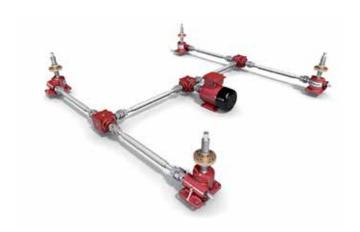
If multiple machine screw jacks are connected in a mechanically linked system then the complete system may be considered self-locking. If you would like this checked consult Power Jacks. Alternatively, to be sure, include a brake on the system either as a stand alone device or as a brake motor.
