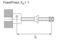
Metric Machine Screw Critical Screw Speed (Shaft Whirling)
