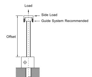
To calculate maximum side load for different raises for screw jacks in tension under full rated load use the following formula to modify the above tabulated values.
