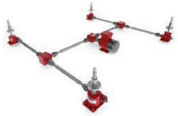
If multiple ball screw jacks are connected in a mechanically linked system then the complete system in some circumstances may be considered self-locking depending on the gear ratios and efficiencies of units in the system. In general, Power Jacks recommend a brake is used on **ALL** Ball Screw Jack systems. If you would like this checked, consult Power Jacks. Alternatively, to be sure, include a brake on the system either as a stand alone device or as a brake motor.
